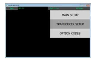
Here you can select the transducer menu and by clicking on the transducer connector port you can move the transducer to the appropriate area of the vessel, and select the transducer, by part number. This will change the parameters to match your transducer.
