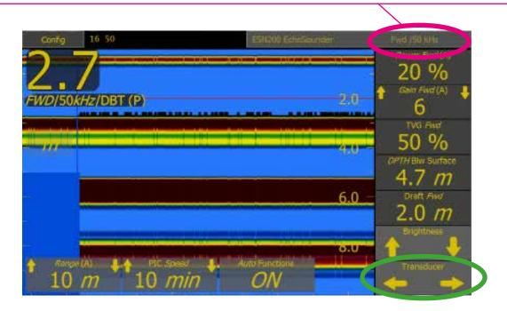
The left right button will allow the user to change the transducer displayed. Each of these may have up to 2 frequencies.
