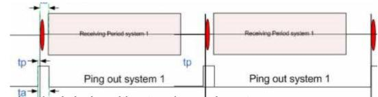
Asynchronised pinging with external acoustic system
