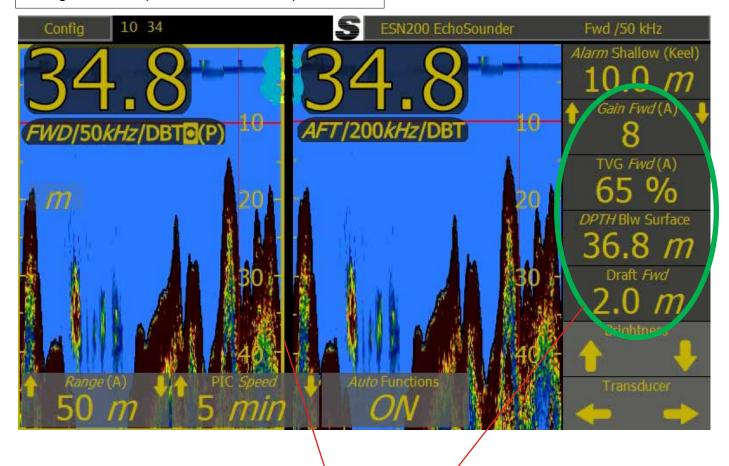
The settings of transducers in the right panel (green circle) is valid for the "Yellow highlighted" channel.(In this example it is the Fwd 50 kHz primary transducer.)
