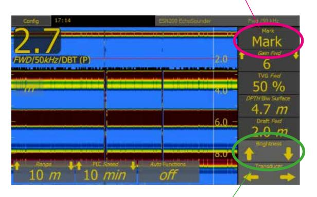
Dimming up and down is available using the up and down arrows, or the slider that pops up when a dimming arrow is touched. IF the system is dimmed too far down, press and hold the screen, and it will return to a 'visible level'.
