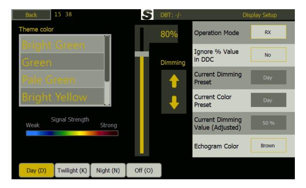
By changing to Day, Twilight, Night, and OFF Text colours can be selected and echogram colour for that level. As the dimming is changed, these colours will change as the dimming level passes through the set level, or if a remote (DDC) command is sent. This allows the user to decide what dimming level is required for this particular display (This may be different in different areas of the Bridge/Control room)
