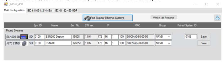
The Connected screens need to be paired to the JB70E2 electronic unit as shown.
