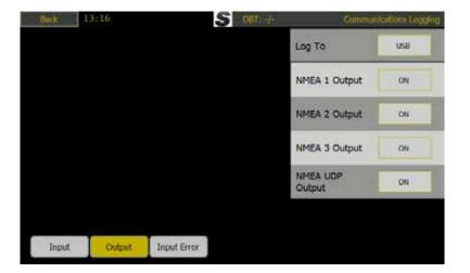
Setup for additional logging of NMEA and/or NMEA UDP to disk
