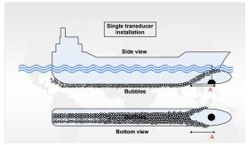
Do not mount transducers close to the propeller or aft of other hull installations (outlets, vents or other protruding details). It is necessary to select a part of the hull that is submerged under all load and speed conditions, and to avoid positions where air is trapped in heavy weather.
