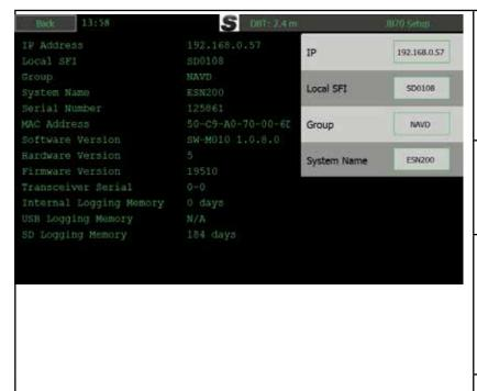
The screen IP can be set up. recommended range is 172.16.1.X, but any private IP address is supported. The IP address must be unique for each unit. The mask is set to 255.255.255.0
