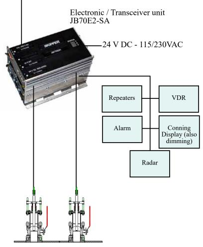
Options for tank, sea valve (single and double hull) and retrofit.
