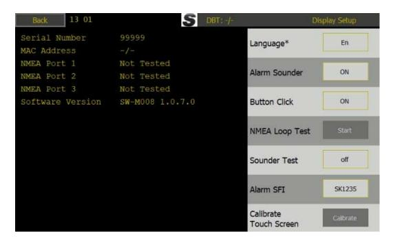
Find software version loaded on the JB70E2 unit Press "Config", "JB70 setup"
